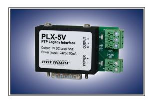
The CYBER SCIENCES PTP Legacy Interface (PLX-5V / PLX-24V) is a wiring adapter for the CyTime<sup>™</sup> Sequence of Events Recorder to output a legacy time protocol to other devices. The adapter fits the "Options" port (DB15 connector) of the SER-3200 or SER-2408 and facilitates wiring of 5V or 24V signals via a screw-type terminal, suitable for power equipment wiring. (Model PLX-5V is shown at left.)
