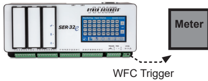
SER, with Trigger Output for Waveform Capture
