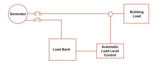
The Automatic Load Level Controller adds and subtracts Load Bank load in response to dynamic power fluctuations in the connected facility load. It utilizes the Load Bank as a "supplemental load" for maintaining a minimum load on the power source.
